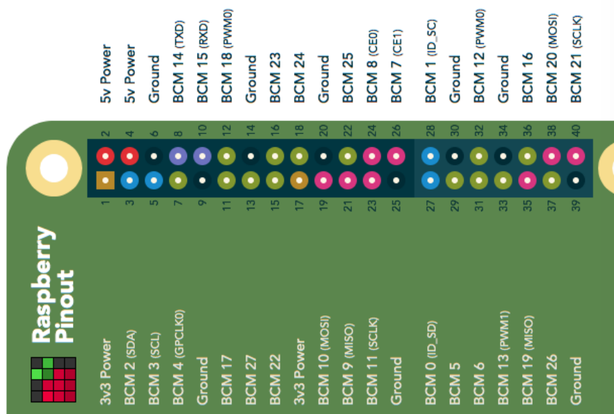
Figure 1.1: Raspberry Pi 2 Pinout 1
