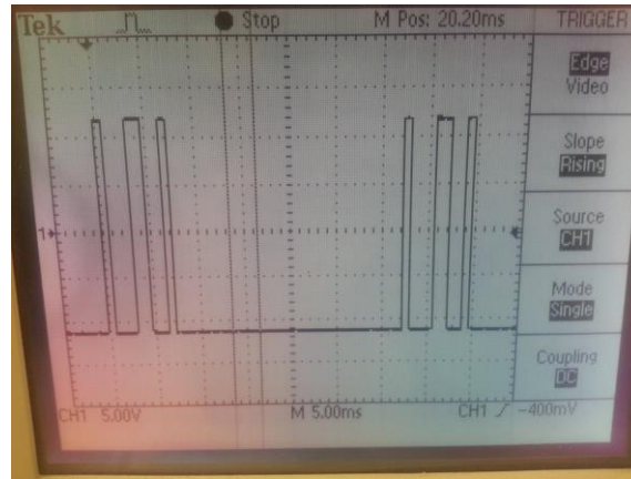
Figure 32. Two ASCII characters being transmitted from the BERT to the DUT using 1200 8N1 RS-232 communication. A 25 ms transmit delay occurs between each ASCII character transmission, but the delay can be reduced. How much of a reduction depends on how quickly the DUT can receive or transmit a single ASCII character.
