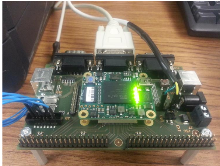
Figure 28. Actual setup of DUT for this senior design project. It is shown interfaced to the BERT (PC; left) via RS-232 serial communication.
