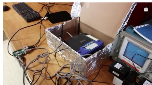
Figure 4.1.1: Com Setup inside Faraday Cage
