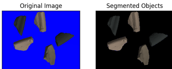
Fig. 8. Sherds in the pickup area before (L) and after (R) color segmentation.
