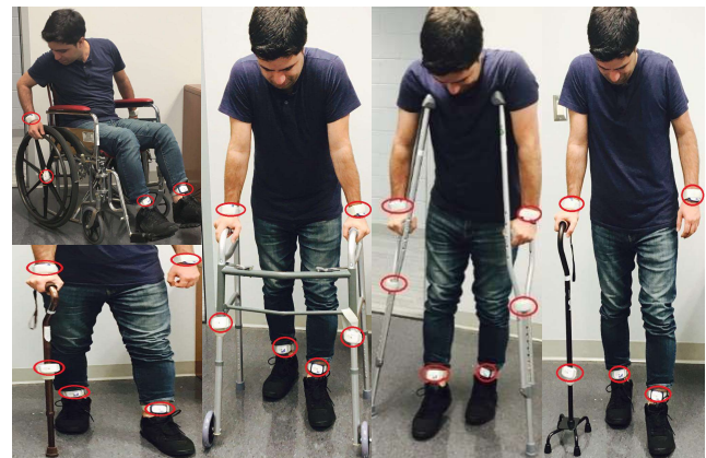
Figure 4: An investigator using various types of mobility aids. Red circles highlight the SenseWear armbands.
