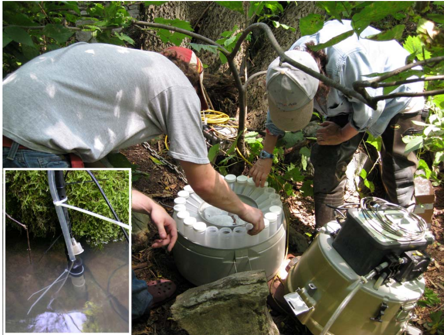
Figure 4: Automatic ISCO stormwater sampler with 24 one-liter bottles used to collected stormwater discharge at the springs. Inset shows water level trigger and pump tubing intake.
