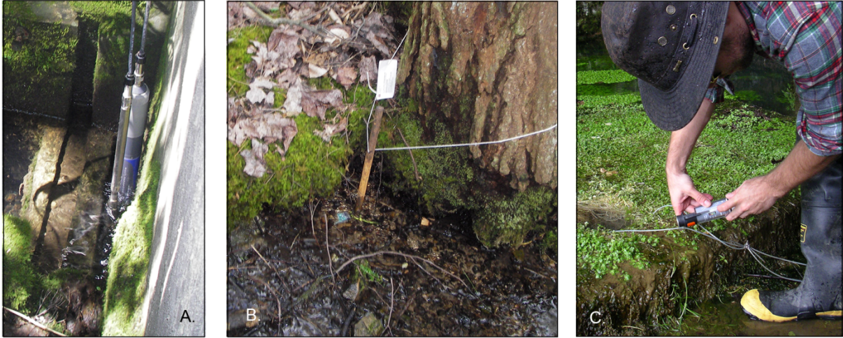
Figure 3: Example of loggers used in recent monitoring. (A) Multiport logger with pH, conductivity, temperature, and water level sensors. (B) Temperature logger attached to a stake. (C) Data download.
