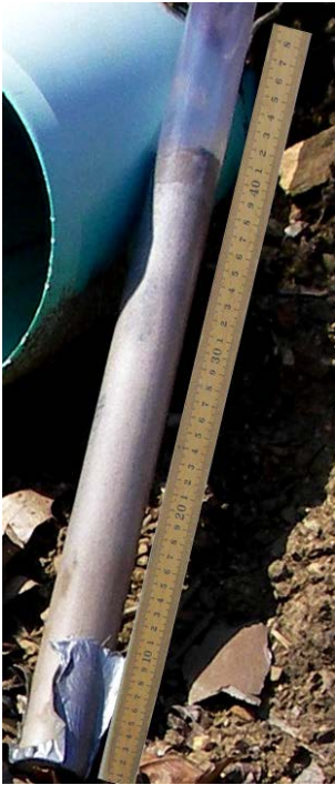
Figure 3: Photograph of core taken from sand trench 18 months after construction showing a layer of fines in the top 2 cm of dark sediment.
