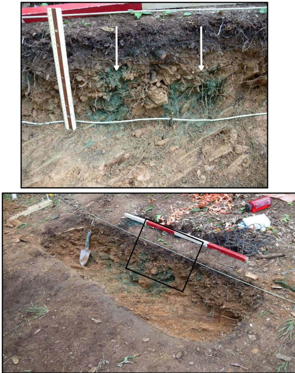
Figure 3: The top photograph shows the excavation face near the center of the injection trench to a depth of 25 cm showing two distinct fingers of dye (arrows). Rope in the photograph shows the intersection of the horizontal and vertical faces. The ruler is 30.5 cm (1 ft) long. The bottom photograph shows the infiltration trench and the final extent of the excavation, reaching a depth of 38 cm. The red and white markings on the pole are each 30.5 cm long. The black box outlines the region photographed in the enlargement above.
