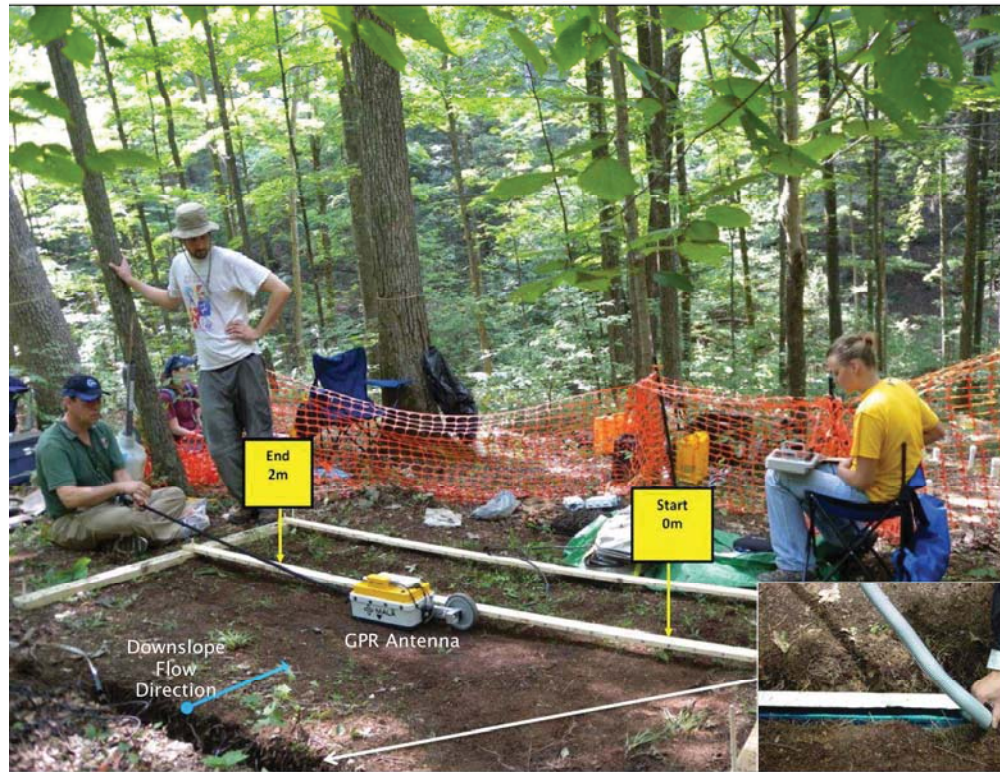
Figure 2: Water and brilliant blue dye were pumped into a shallow trench upslope of the GPR survey grid. A slotted, meter-long PVC pipe (inset) was used to ensure the tracer solution was dispersed uniformly and to maintain a constant head during the injection. An adjustable wooden frame acted as a GPR antenna guide to ensure reproducible data collection.
