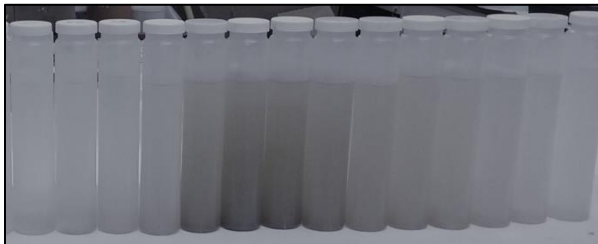
Figure 4. Visual turbidity change in Tipperly Spring water samples capturing the storm pulse as it reached the spring. Increased turbidity resulted in darker bottles and therefore a lower pixel luminosity. Shown: May storm samples from 5/5/17 6:00-20:00.
