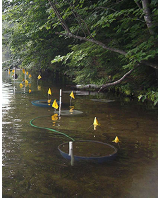
Figure 6: Photograph of an array of seepage meters on the southwest shore of Mirror Lake, NH. The seepage meter is a half-barrel inserted into the bed sediments with a bag attached by a hose. The bag is protected from waves by a bag shelter. Mini piezometers are driven into the lake bed nearby to measure the difference in head between the groundwater and the lake.
