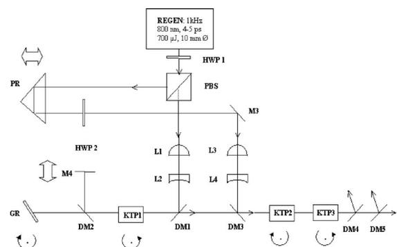
FIG. 4. Layout of the optical parametric amplifier: (HWP) half-wave plate, (PBS) polarizing beamsplitter, (L) lens, (M) silver mirrors, (DM) dichroic mirrors, (KTP) nonlinear crystals, (GR) grating, (PR) prism.
