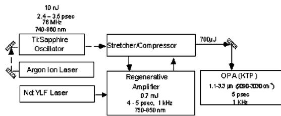
FIG. 2. Diagram of the Ti:sapphire regenerative amplifier and optical parametric amplifier. The Ti:sapphire oscillator pumped by an Ar ion laser provides 2.4–3.5 ps pulses with 10 nJ/pulse energy at 76 MHz repetition rate tunable 740–860 nm. Regenerative amplifier pumped by a Nd:YLF laser amplifies pulses to 0.7 mJ/pulse energy at 1 kHz repetition rate. The output of the amplifier is sent to the optical parametric amplifier for frequency conversion to the infrared.
