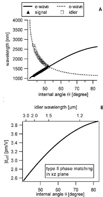
FIG. 1. Theoretical and experimental tuning curve (A) and theoretical values of effective nonlinearity  $d_{\text{eff}}$  (B) for type II phase matching in the KTP  $xz$  plane. On the phase matching curve (A), the circles are measured signal ( $e$ ) wavelength and squares are measured idler ( $o$ ) wavelength. The  $o$  wave denotes ordinary wave,  $e$  wave denotes extraordinary wave. The line is the calculated phase matching angles.
