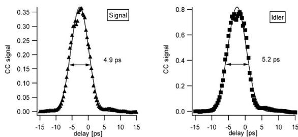
FIG. 8. Crosscorrelation of signal and idler pulses. Solid line is Gaussian fit. FWHMs are 6.4 and 6.8 ps; corresponding pulse duration are 4.9 and 5.2 ps for signal and idler pulses, respectively.
