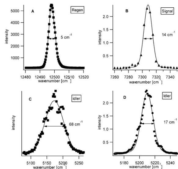
FIG. 7. Bandwidth of pump and signal, idler wavelength: (A) spectra of pump. Bandwidth of pump is 5 cm<sup>-1</sup>, (C) bandwidth of idler when there is no grating in OPA. In this condition idler bandwidth is 68 cm<sup>-1</sup>. For comparison, (B) and (D) show signal and idler bandwidth with 1200 gr/mm (blazed at 1  $\mu$ m) grating in OPA. Signal and idler bandwidths are 14 and 17 cm<sup>-1</sup>, respectively.
