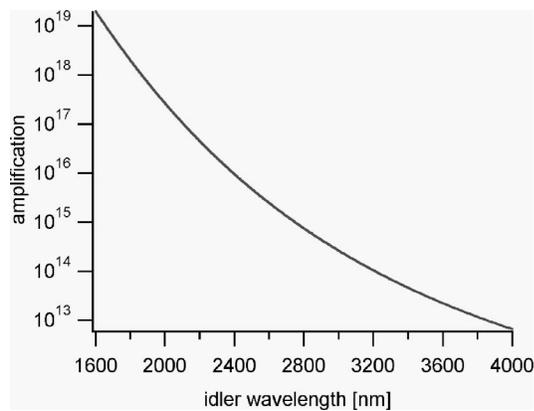
FIG. 6. Estimated amplification for KTP type II phasematching in the  $xz$  plane. Calculation is based on Eqs. (3) and (4) taking pump power 25 GW/cm<sup>2</sup>, crystal length 1 cm.
