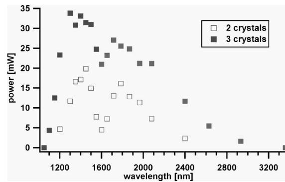
FIG. 5. Signal ( $\lambda < 1600$  nm) and idler ( $\lambda > 1600$  nm) power as a function of wavelength. Open squares were measured with a two-crystal configuration, filled squares with a three-crystal configuration.
